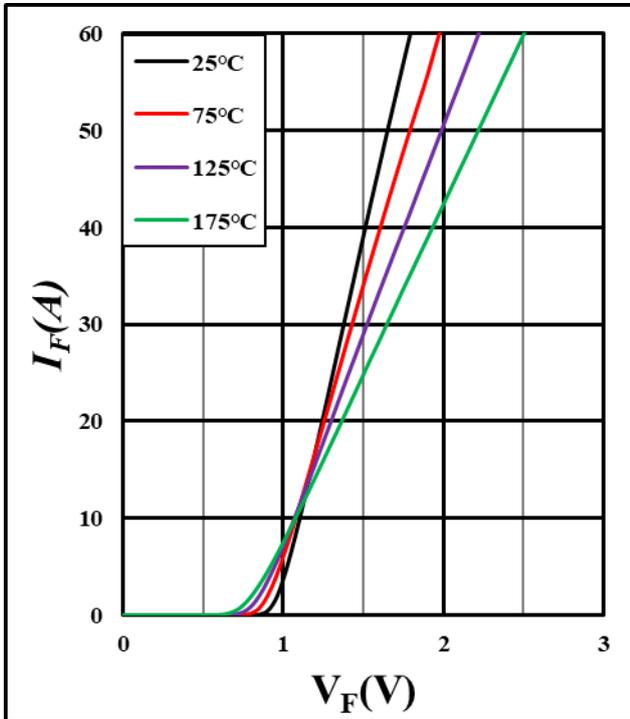
Figure 1. Forward characteristics
