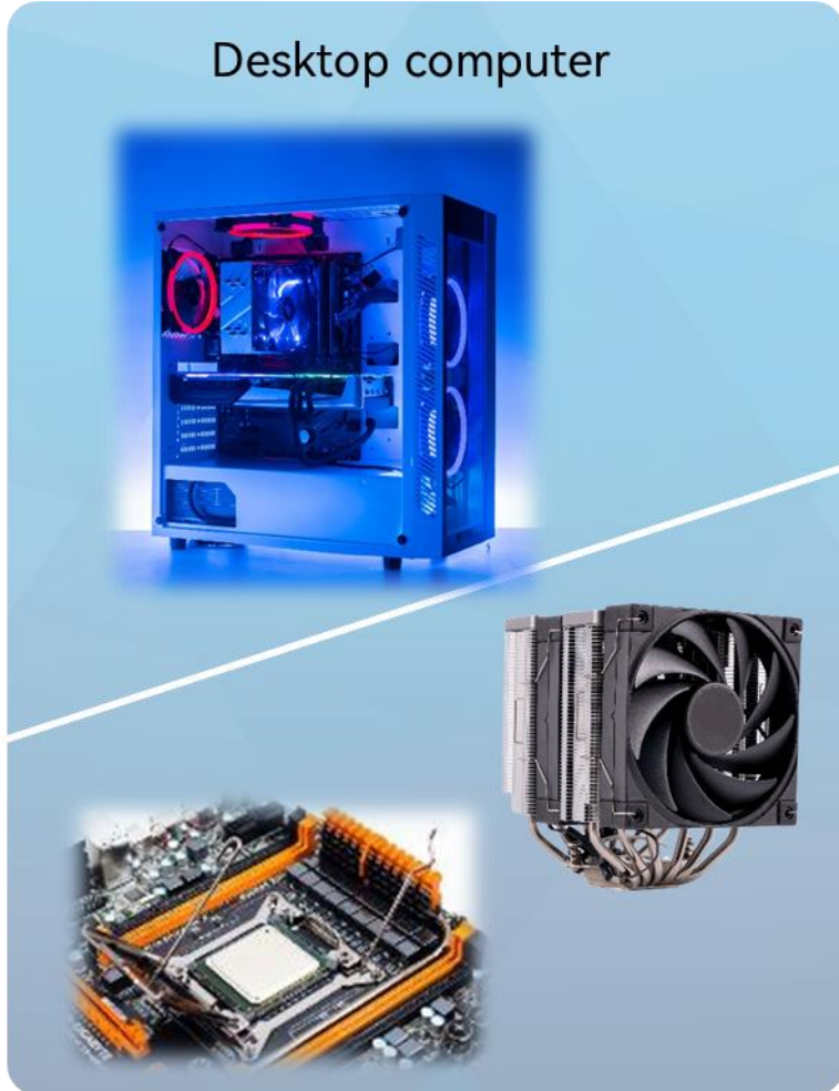
High-power CPU cooled by cooling tower
