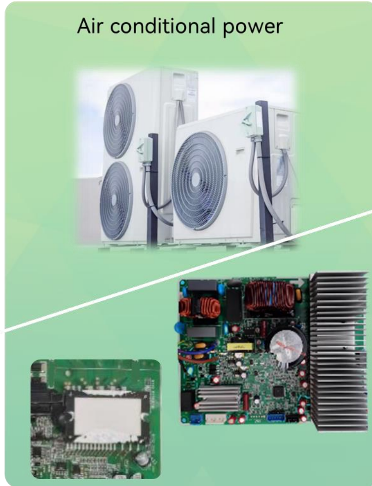
Air Conditional inverter IPM module with aluminum heat-sink
