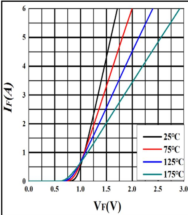
Figure 1. Forward characteristics
