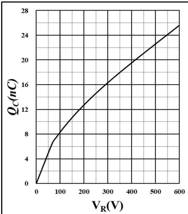
Figure 7. Total capacitance charge vs. reverse voltage
