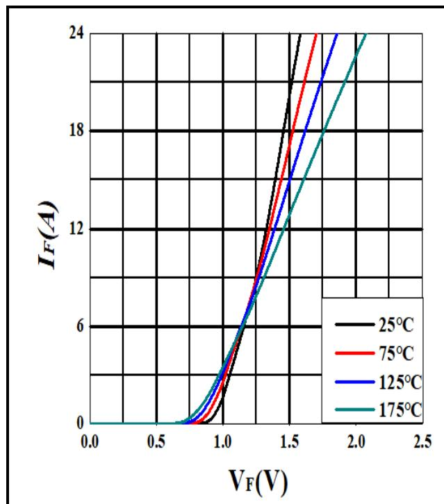
Figure 1. Forward characteristics
