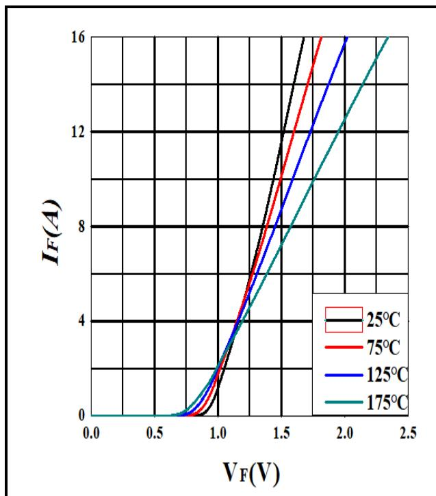
Figure 1. Forward characteristics
